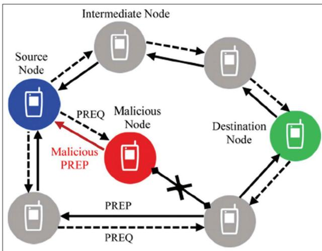
**Figure 3:** Mobile *ad hoc* network's black hole attack
