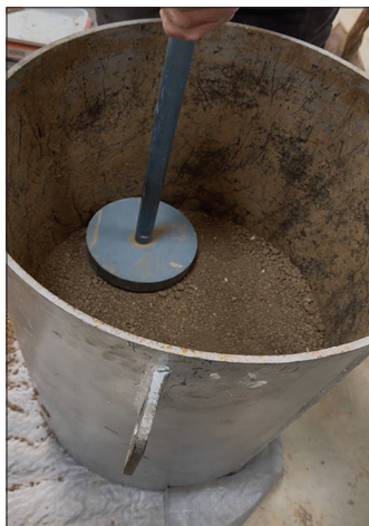
Figure 6: Compaction of soft soil
