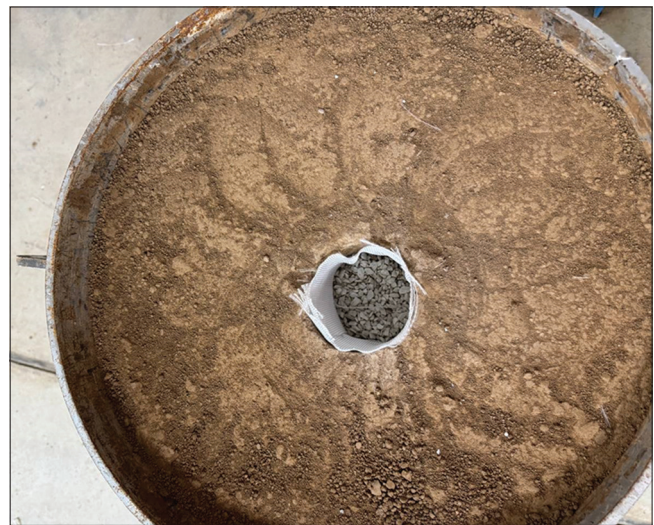
Figure 7: Geotextile and crushed stone aggregate
