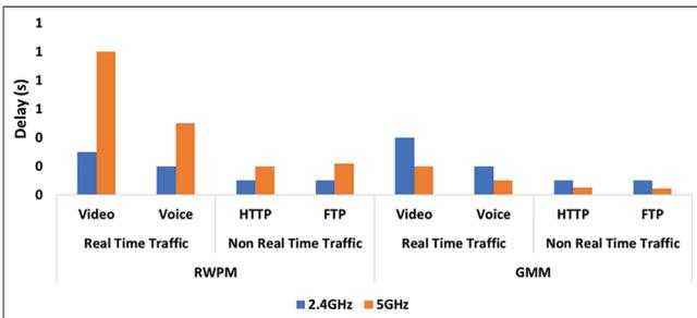
**Figure 8:** Average delay for real-time and non-real-time traffic
