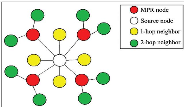
Figure 5: MPR's nodes of OLSR routing protocol<sup>[13]</sup>
