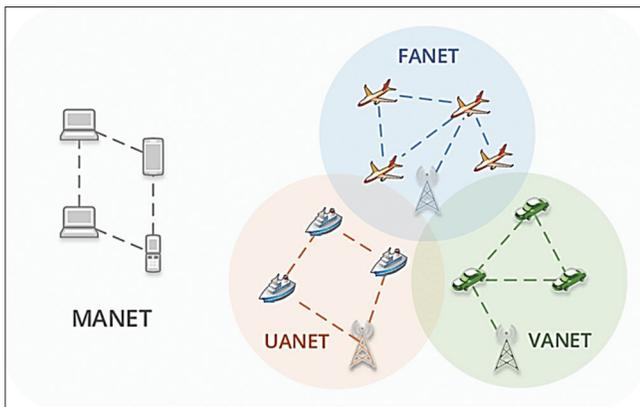
Figure 1: Different types of mobile ad hoc networks<sup>[2]</sup>
