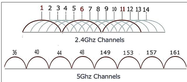
Figure 3: Different types of channels of 2.4 GHz and 5 GHz<sup>[11]</sup>
