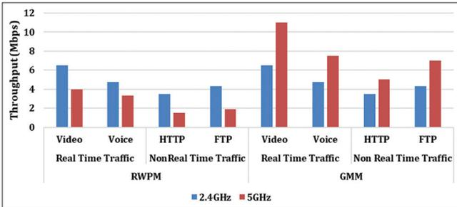
**Figure 7:** Average throughput for real-time and non-real-time traffic
